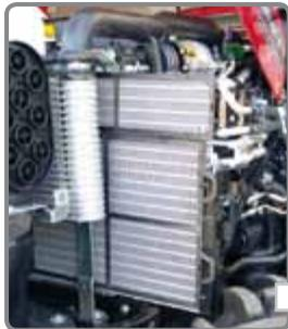
Quantum engines are equipped with turbocharger and an air to air intercooler to boost thermal efficiency and extract maximum power from every drop of fuel. **Quantum engines allow easy access for cleaning and servicing.**
