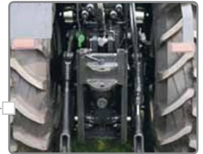
**More flexibility with hydraulic stabiliser struts** easily controlled from inside the cab.
