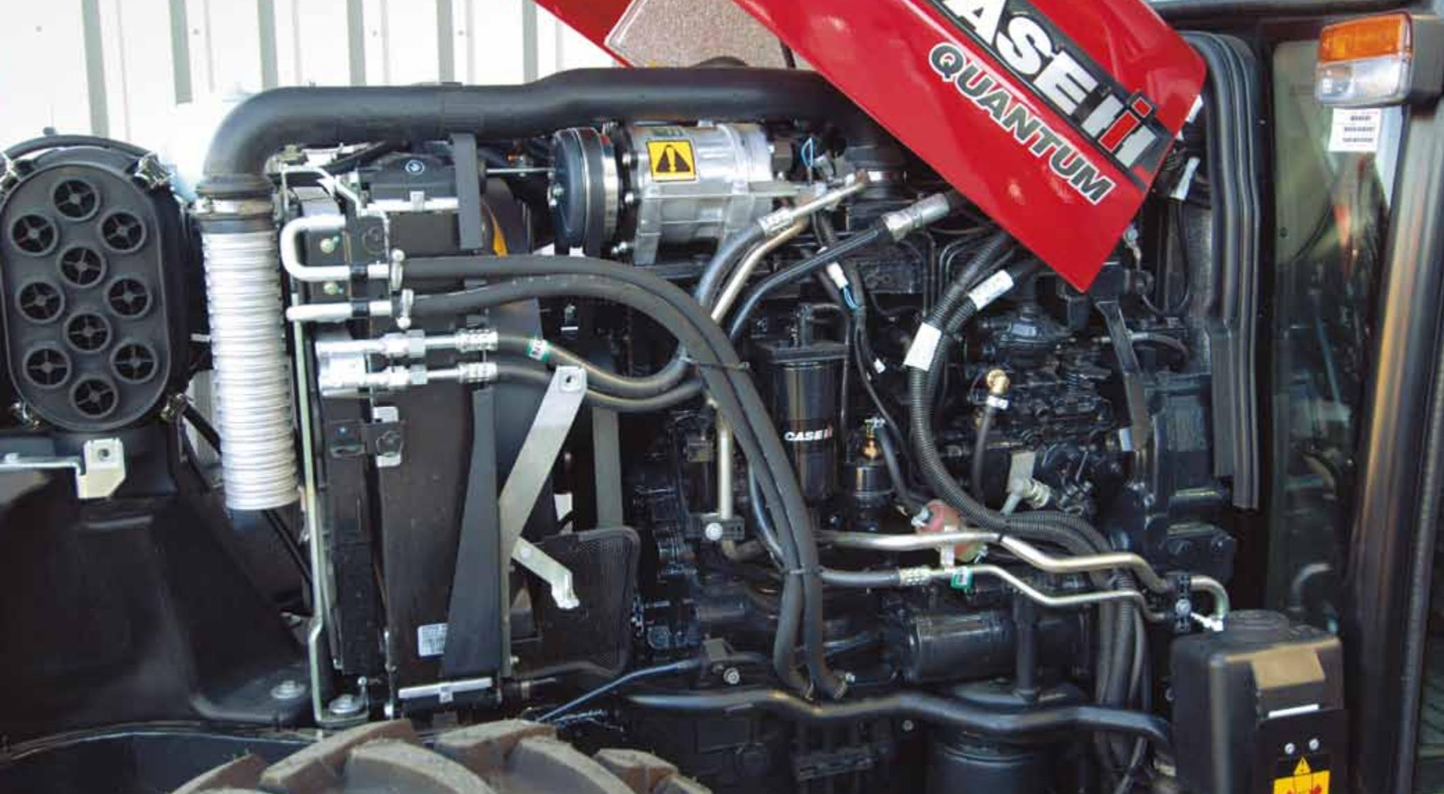
**Low clearance.** The horizontal exhaust system allows these tractors to easily operate under overhanging branches. An optional vertical exhaust is available for cab models.
